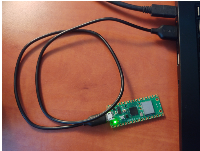
Figure 4.1: A picture of a Raspberry Pi Pico W (the green board) connected to the computer.
