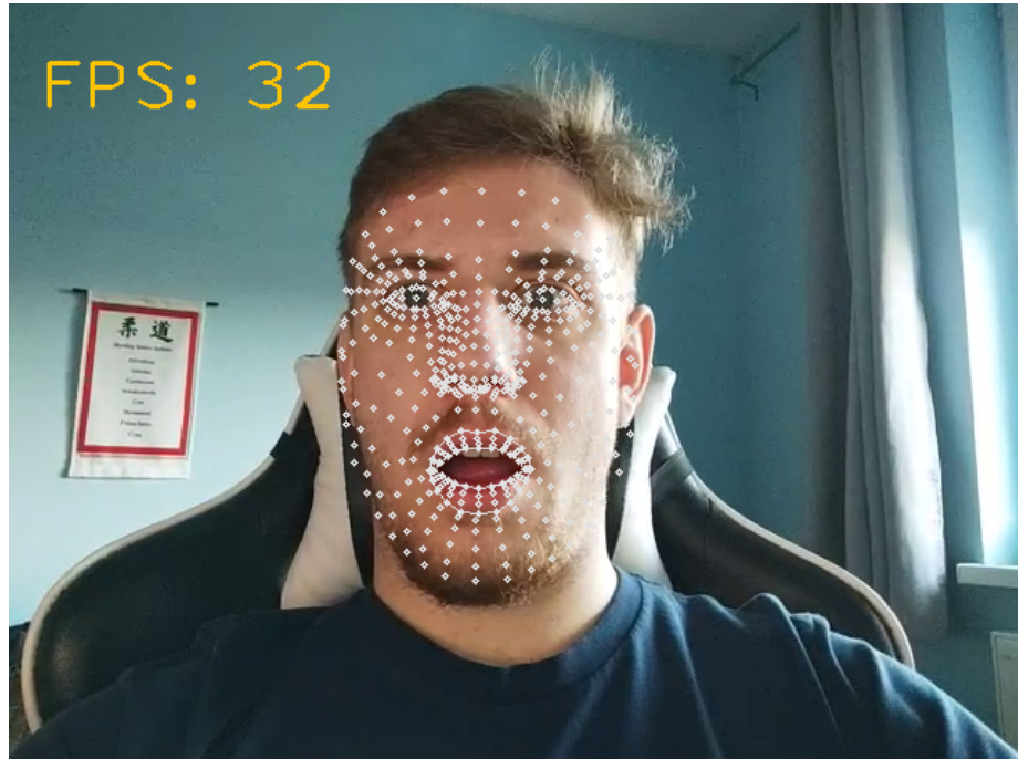
Figure 4.1: The resulting window of Face tracking module consists of the input frame, calculated landmarks, and inference speed.
