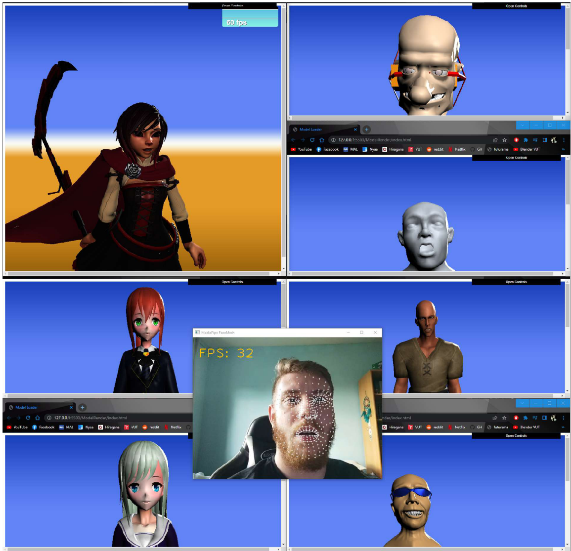
Figure 4.5: Test showing both camera FPS (32) and rendering FPS (60+), while rendering 7 different avatars.
