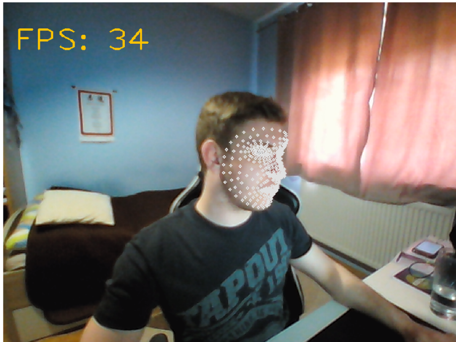
Figure 2.5: Facemesh produces 478 landmarks, which define the face geometry, even under difficult angle and light conditions
