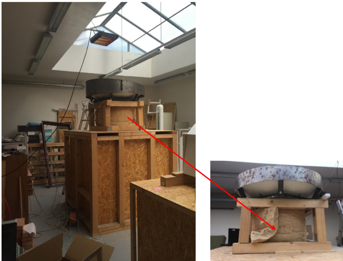
Fig. 4.3: Photograph of the light guide with additional thermal insulation (mineral wool)
