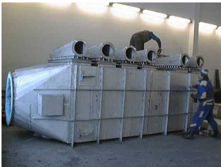
Figure 2.12. Made-to-measure heat exchanger for preheating of fluidizing and combustion air (Stehlík, 2011, reprinted with permission of EVECO Brno, Ltd.)
