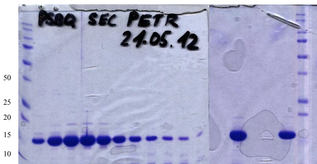
Figure 14: A - SDS-PAGE of Size Exclusion Chromatography, B - concentrated fractions (left 20\mu\text{L} , right 15\mu\text{L} of sample)
