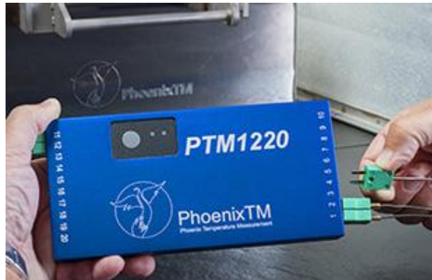
Fig. 14: Datalogger Phoenix, a version PTM1220. Taken from [39]
