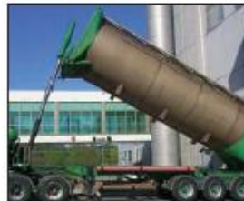
Emptying silo vehicles
