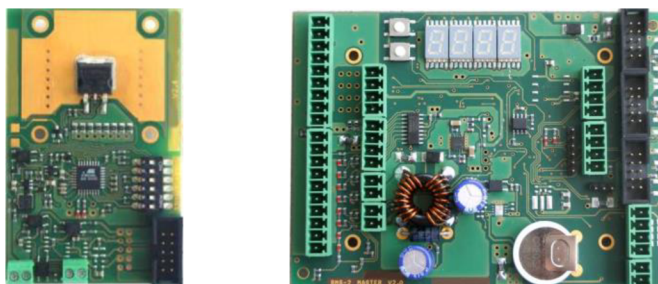
Obr. 47 Modul CBU a Master RT-BMS CU.
