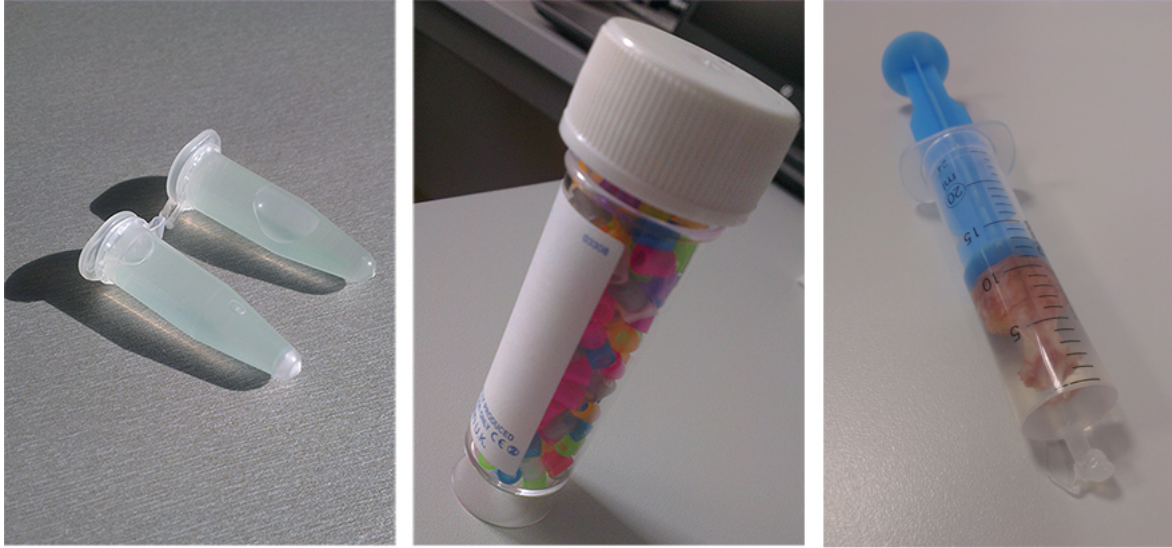
Figure 8.1: Phantoms used for measurement. The TTP phantom (left), the PBP phantom (middle), and the isolated rat brain in cranium (right).
