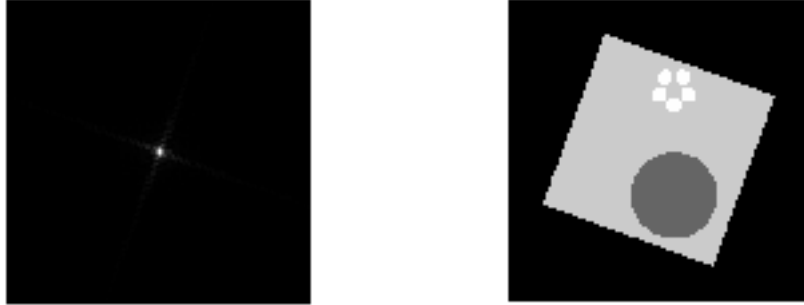
Figure 7.3: Template of phantom used for testing quality of reconstruction. Original cartesian k-space data (left), zoom 5x. 2D IFFT of the k-space data (right).
