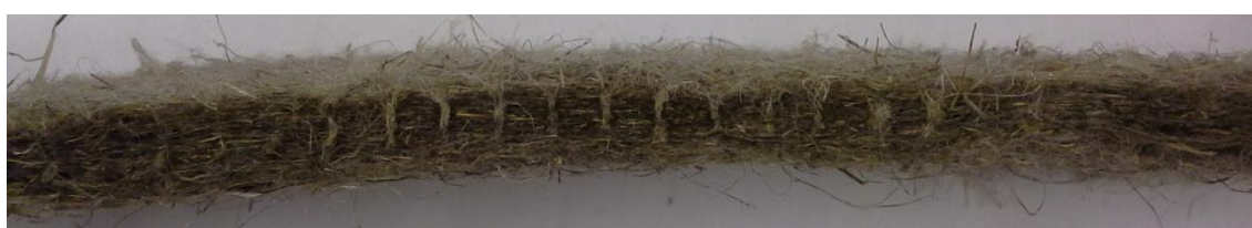
Figure 20 Section of a reinforced mat
