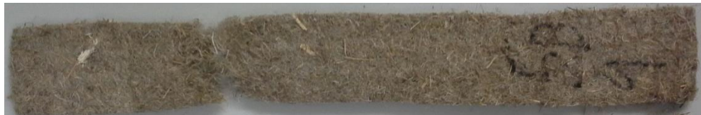
Figure 46 Specimen broken at low load
