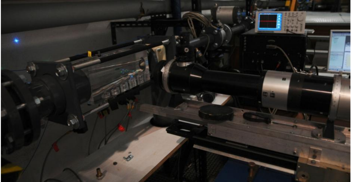
Figure 14 Overall view of LDA measurements
