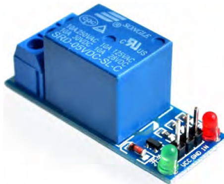
Obr. 6.1: Relé Songle SRD-xxVDC-SL-C [18]
