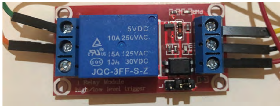
Obr. 6.2: Relé Tongling JQC-3FF-S-Z
