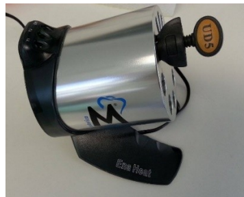
Figure 60: Shows the resin composite heater used in group 3
