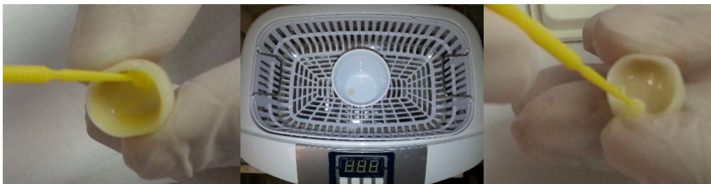
Figure 45: Shows the application of hydrofluoric acid, ultrasonic cleaning with alcohol, and silane application to prepare the ceramic surface
