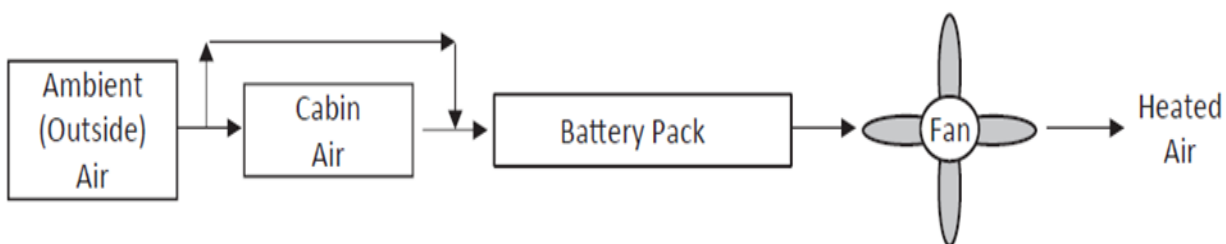
Figure 5 : Passive air cooling schematic [8]
