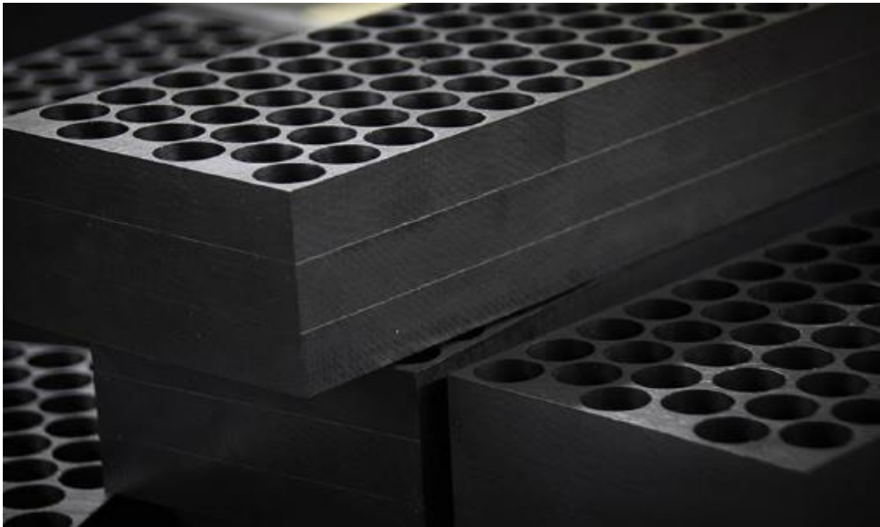
Figure 8 : All cell phase change composite (PCC™) material [8]
