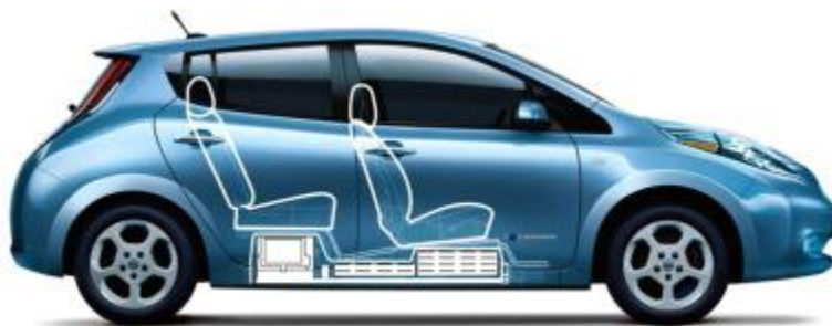
Figure 12 : Placement of lithium ion battery pack in Nissan Leaf [15]
