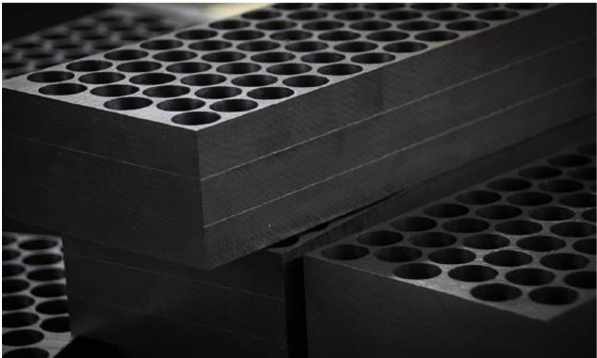
Figure 8 : All cell phase change composite (PCC™) material [8]
