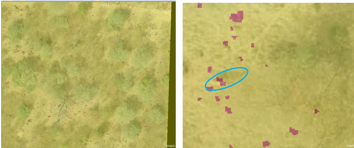
Figure 13: Output of 8 treatment (left) and one of two detected WDE (in blue oval) surrounded by several “false positives” (right)
