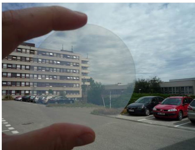
Figure 25: Transparent zirconia-doped TM-DAR + Z(24) disc (80 mm diameter and 0.8 mm thickness) [47].
