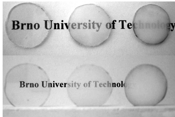
Figure 26: The optical transparency of spinel ceramics (thickness 1.1mm) prepared with different presintered densities (from left: 94.9, 97.9 and 99.5 %t.d.). In the upper image the samples are lying immediately on the sheet of paper bearing the text; in the lower one they are 5 cm above it [50].
