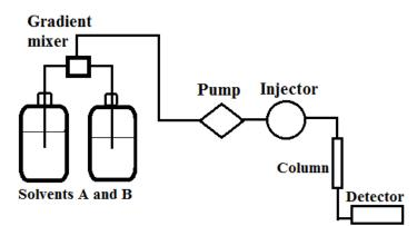
Figure 6: Simplified HPLC instrumentation (gradient system)
