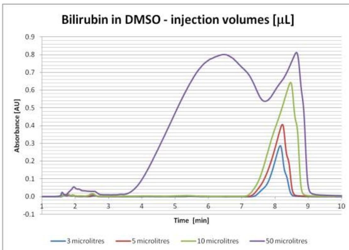
**Figure 7:** Influence of injection volume, mobile phase: methanol-acetonitrile-2% acetic acid (75:22.23:2.67) and the column: Agilent Zorbax SB-C18: 4.6 mm ID × 150 mm, (5 µm)
