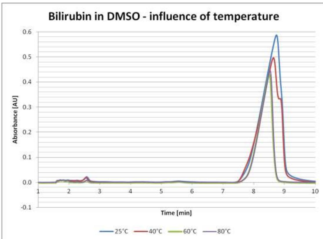
**Figure 8:** Influence of the temperature, mobile phase: methanol-acetonitrile-2% acetic acid (75:22.23:2.67) and the column: Agilent Zorbax SB-C18: 4.6 mm ID × 150 mm, (5 µm), injection volume: 5 µL
