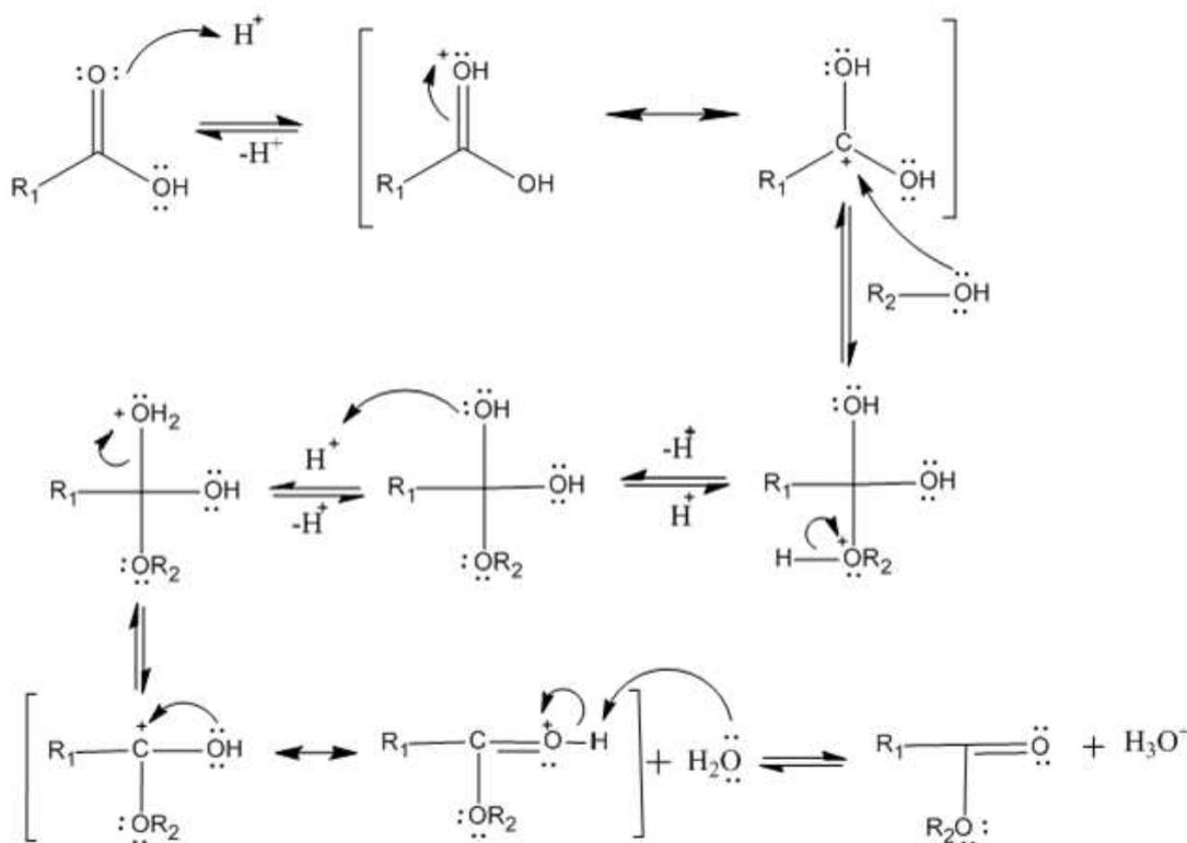
**Figure 4:** Reaction mechanism of the Fischer esterification
