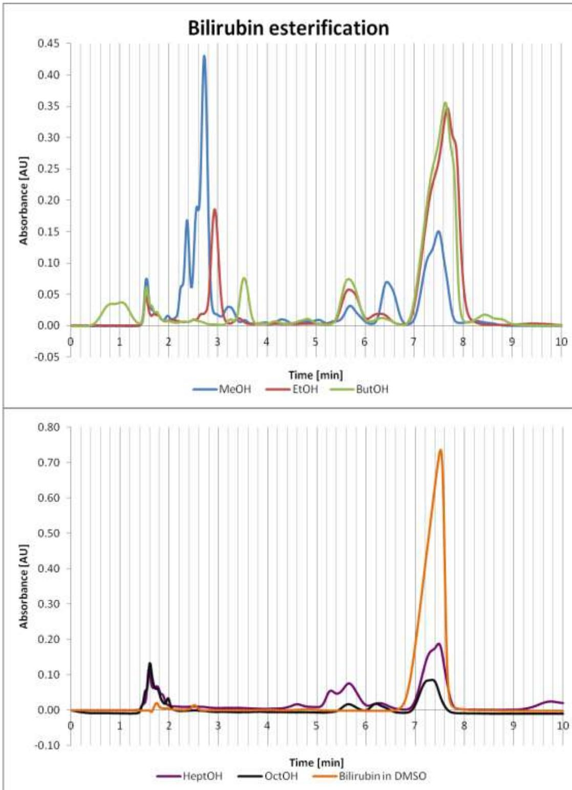
**Figure 11:** Bilirubin dissolved in DMSO, mixed with alcohol in ratio 1:1, acidity: 2% H<sup>+</sup>, column: Agilent Zorbax SB-C18: 4.6 mm ID × 150 mm, (5 μm), mobile phase: CHINA, injection volume: 5 μL
