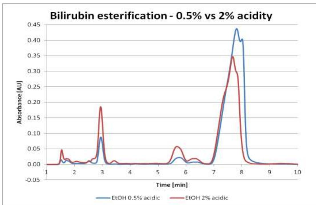
**Figure 12:** Bilirubin dissolved in DMSO, mixed with alcohol in ratio 1:1, acidity: 2%  $H^+$ , column: Agilent Zorbax SB-C18: 4.6 mm ID  $\times$  150 mm, (5  $\mu$ m), mobile phase: CHINA
