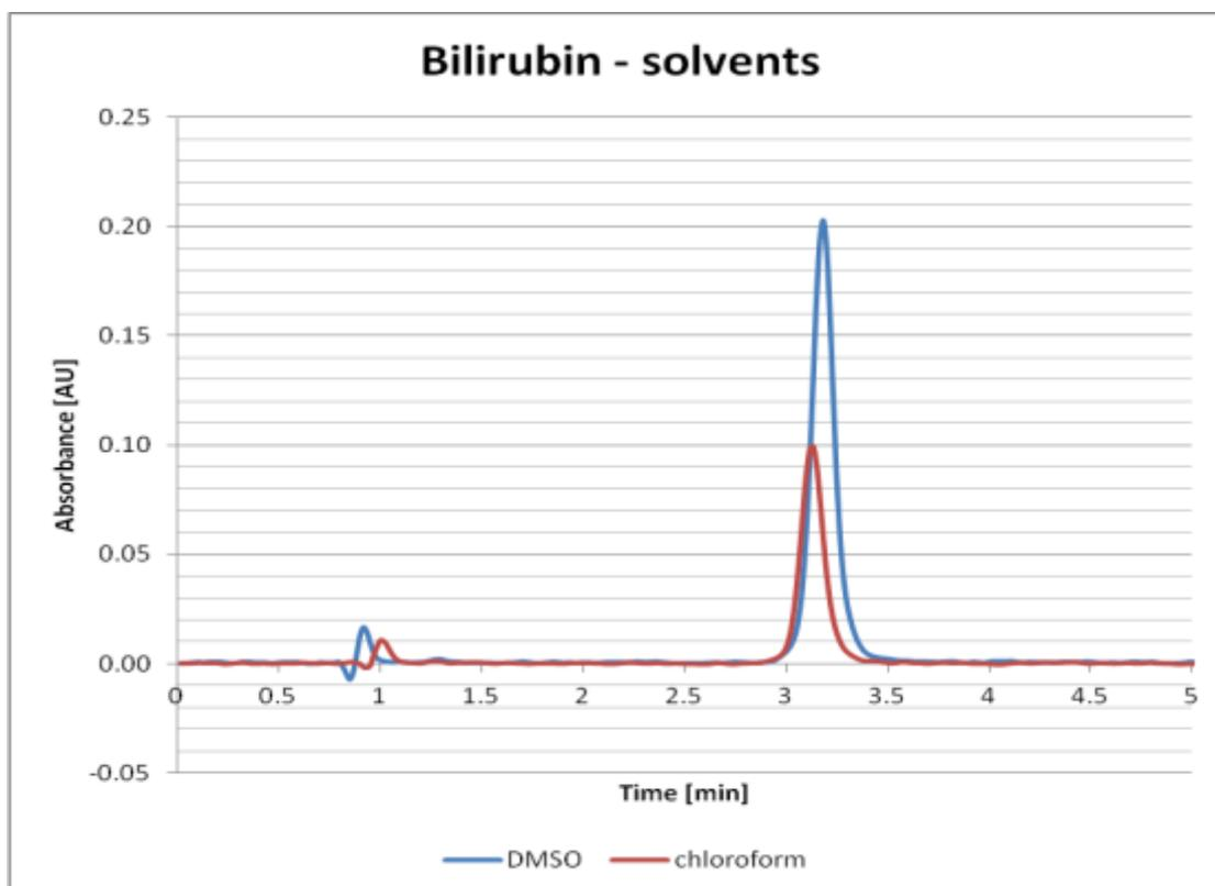
**Figure 9:** Solvents DMSO vs chloroform, mobile phase: CHINA and the column: Waters Symmetry C18: 4.6 mm ID × 75 mm, (3,5 μm), injection volume: 3 μL
