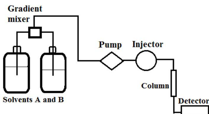
**Figure 6:** Simplified HPLC instrumentation (gradient system)
