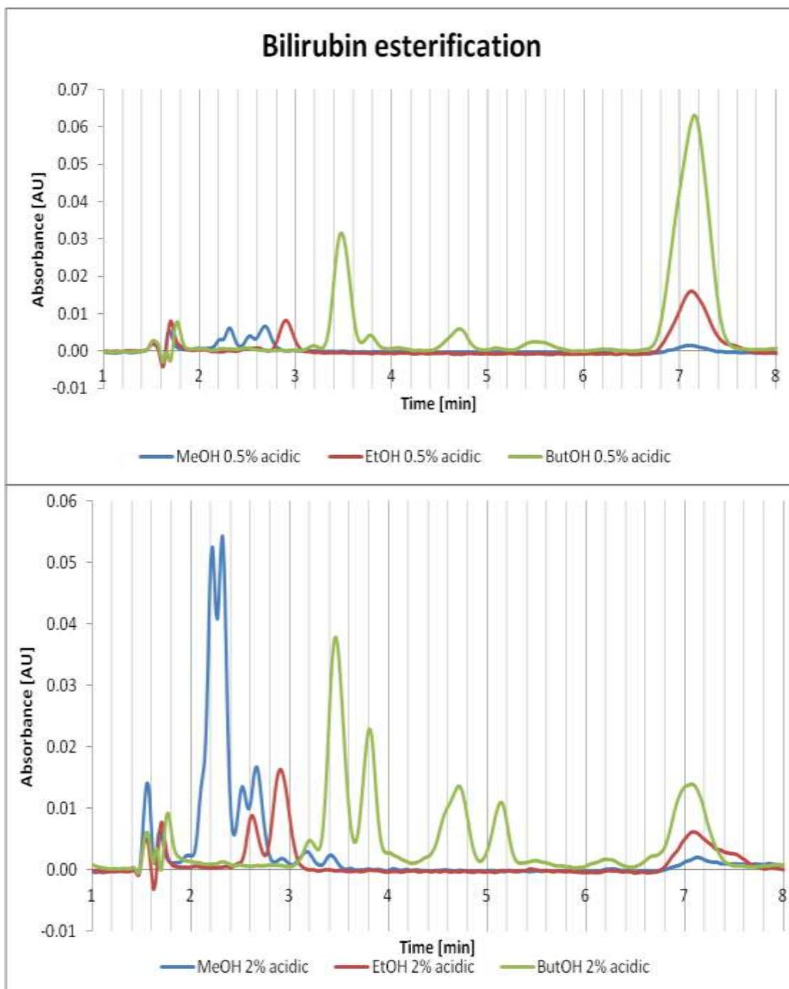
**Figure 13:** Bilirubin dissolved in DMSO, mixed with alcohol in ratio 2:8, acidity: 2%  $H^+$ , column: Agilent Zorbax SB-C18: 4.6 mm ID  $\times$  150 mm, (5  $\mu$ m), mobile phase: CHINA
