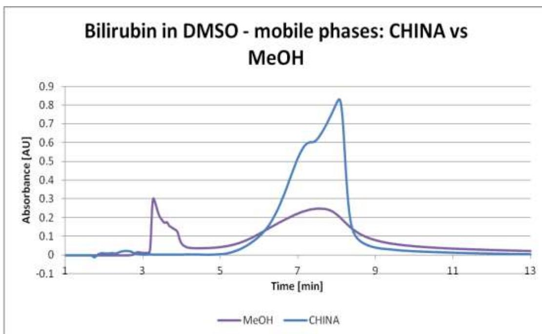
**Figure 10:** Column: Agilent Zorbax ODS: (C18) 4.6 mm ID  $\times$  200 mm, (5  $\mu$ m), injection volume: 50  $\mu$ L
