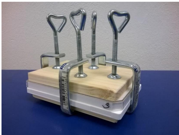
Figure 11. The plates and the lids fastened by handmade wooden pads and clamps to enhance fixation (Houdkova 2017)
