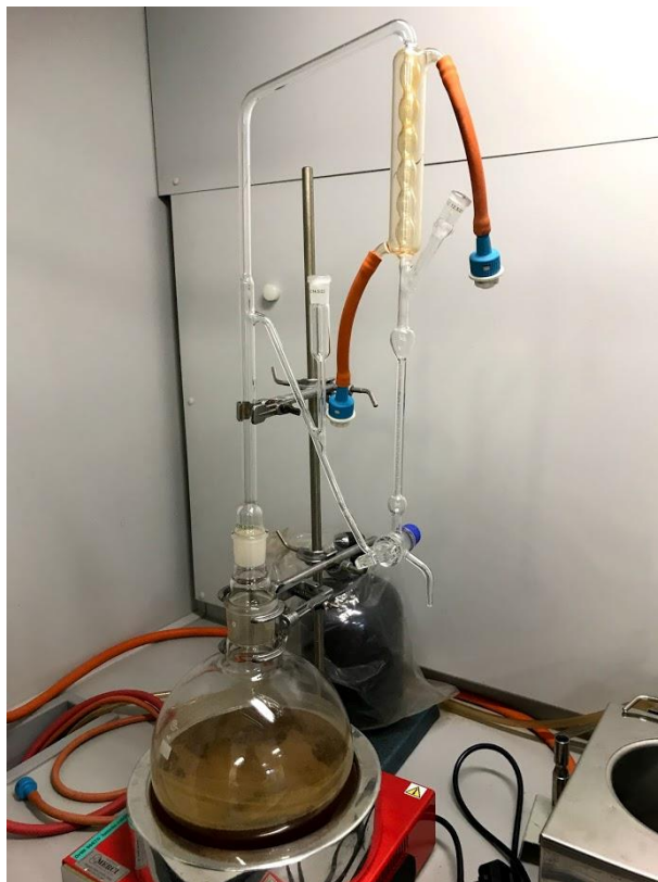
Figure 5. Clevenger apparatus (Merci, Brno, Czech Republic) (Tůmová 2021)
