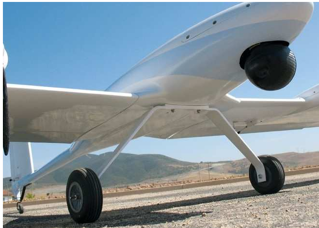
Fig. 4.4 Landing gear type [14]
