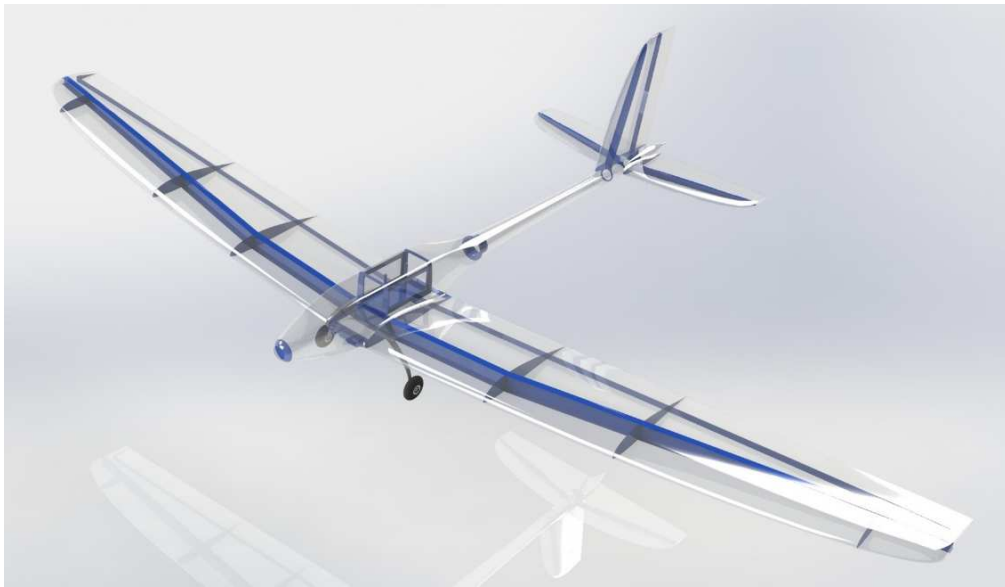
Fig. 8.1 UAV internal structure
