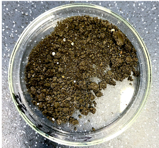
Figure 27: The chernozem soil originally containing 3% of P3HB after 9 months of degradation.
