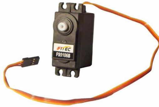
Figure 22 – The FS5106B servomotor from Fitec. Source: (Scarpino, 2015)
