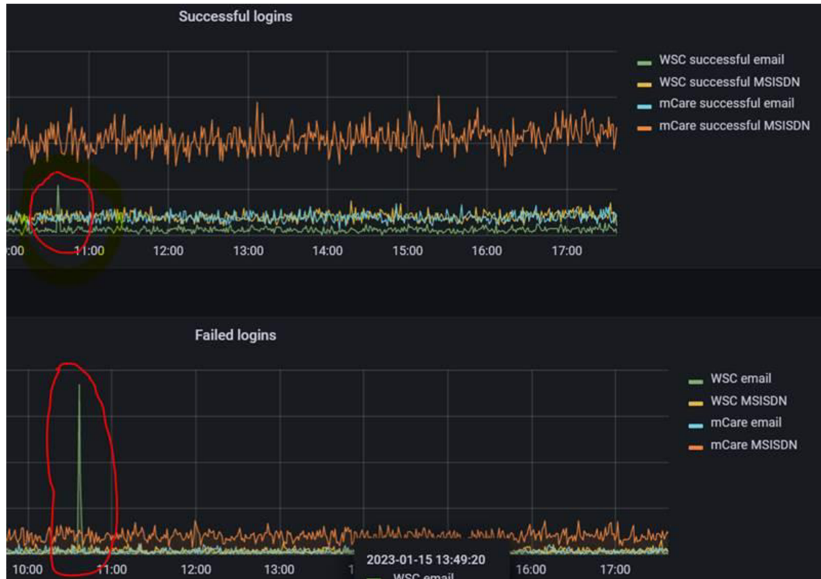
Figure 16: Visuals of Account Hijack - Brute Force - Credential Stuffing Attack by Multiple IPs (Source: Author)
