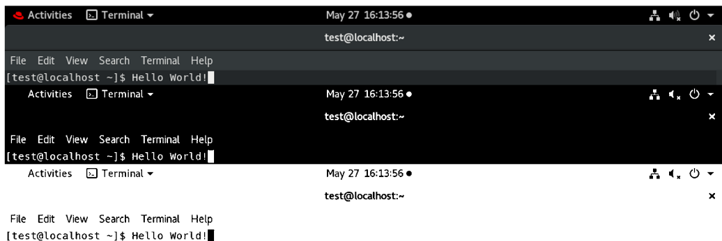
Figure 4.5: Steps of image preprocessing for the OCR, from the top: the original image, the binarized image, the inverted binarized image
