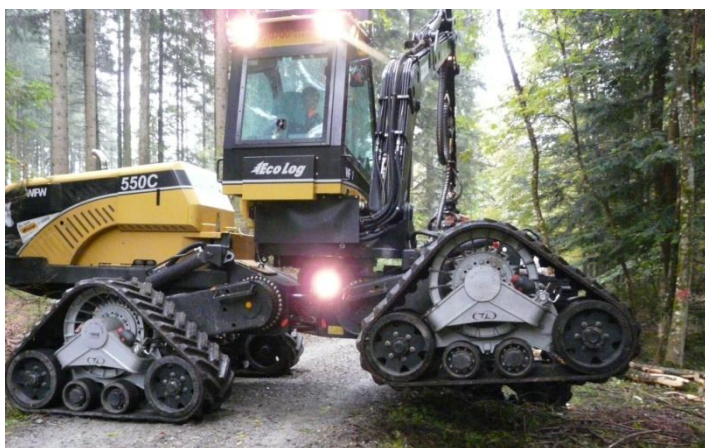
Obr. 12 Harvester EcoLog 550C s pásy Tidue 24D18 [17]
