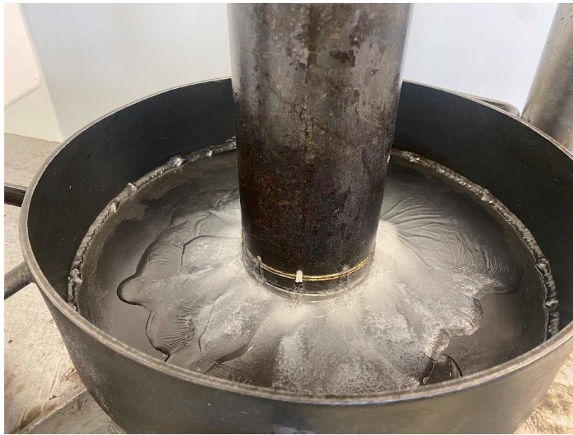
Appendix 3. Compression test of sample at 60 °C showing the output oil.
