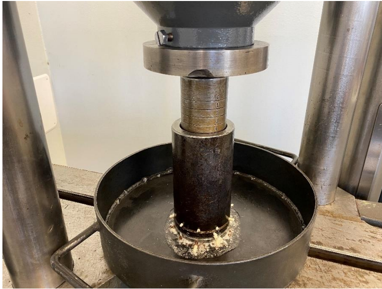
Appendix 1. Compression test of sample at 20 °C (control temperature) showing the output oil.
