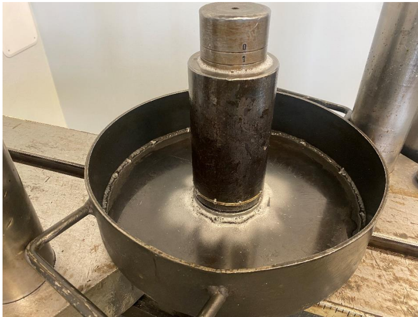
Appendix 5. Compression test of sample at 100 °C showing the output oil
