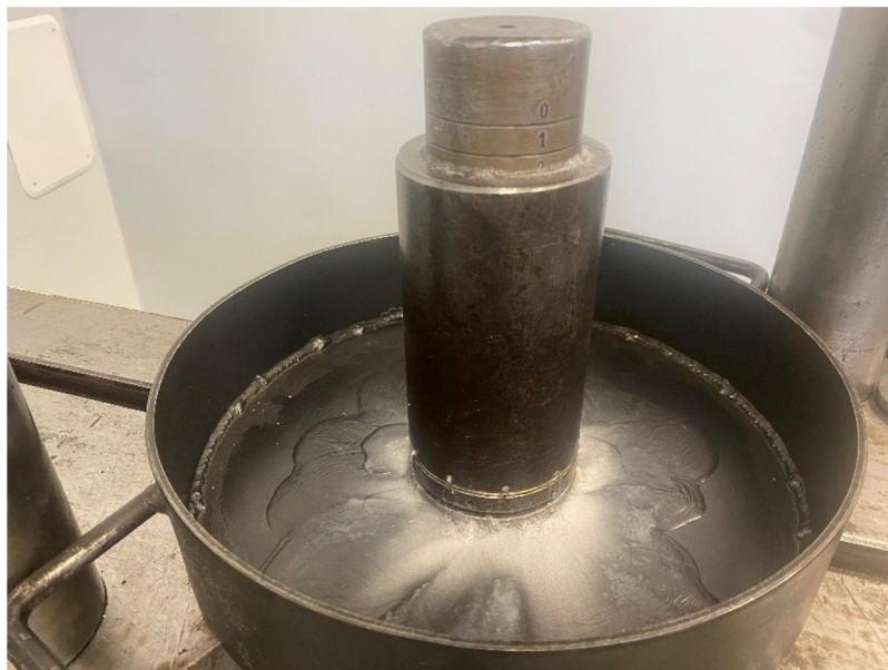
Appendix 4. Compression test of sample at 80 °C showing the output oil.
