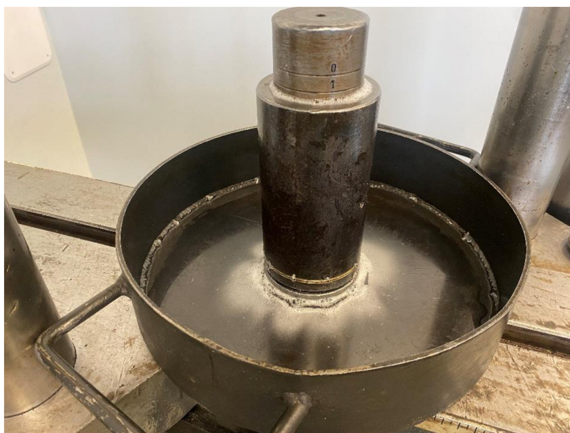
Appendix 5. Compression test of sample at 100 °C showing the output oil
