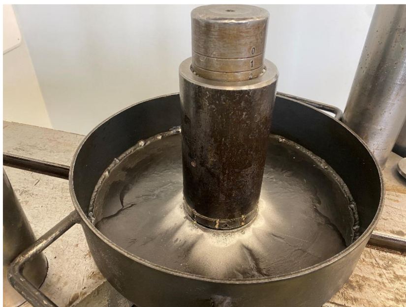
Appendix 6. Compression test of sample at 120 °C showing the output oil.
