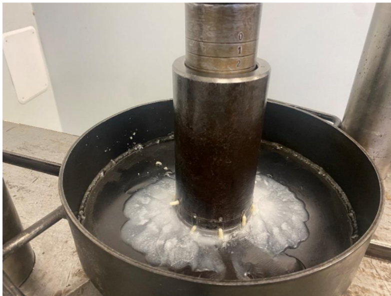
Appendix 2. Compression test of sample at 40 °C showing the output oil.
