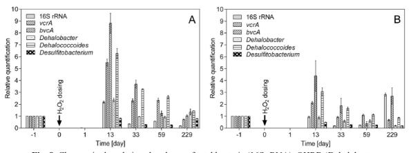
**Fig. 8.** Changes in the relative abundance of total bacteria (16S rRNA), OHRB (Dehalobacter, *Dehalococcoides*, and *Desulfitobacterium*), and VC reductase genes (*vcrA* and *bvcA*) following H<sub>2</sub>O<sub>2</sub> application in well RW5-11: A) depth 8 m, B) depth 13 m. No molecular genetic markers were detected one day after dosing.
