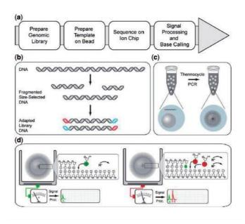
**Fig. 6.** Whole-genome sequencing workflow on Ion Torrent platform. (a) The overall workflow. (b) A genome library preparation. (c) Clonal amplification. (d) Sequencing on the chip. Modified from (Golan and Medvedev, 2013).
