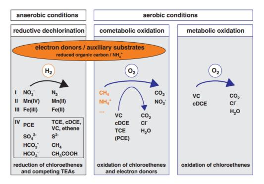
**Fig. 2.** Comparison of reductive dechlorination with cometabolic and metabolic oxidation in terms of the need for auxiliary substrates as electron donors and competing reactions. TEA: terminal electron acceptor. The numbers indicate the order of the different respiration processes (Tiehm and Schmidt, 2011).
