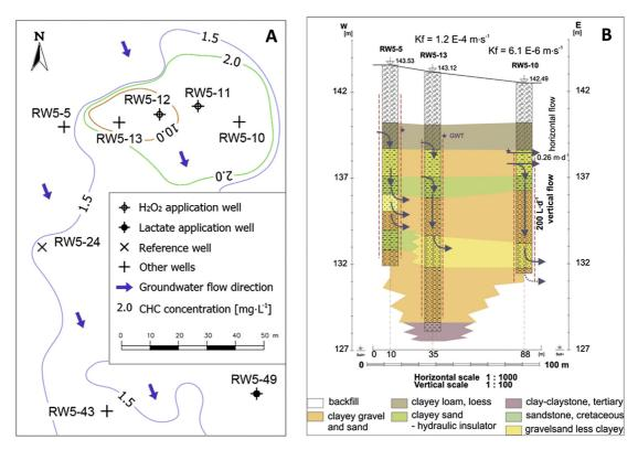
Fig. 1. A) Location of sampling and reference wells, including wells (RW5-5, RW5-10 and RW5-13) illustrating cross-section at the Spolchemie site (Ústí nad Labem, Czech Republic); and, B) geological cross-section of the site showing the open casings of the wells and direction of water flow (blue arrows).
