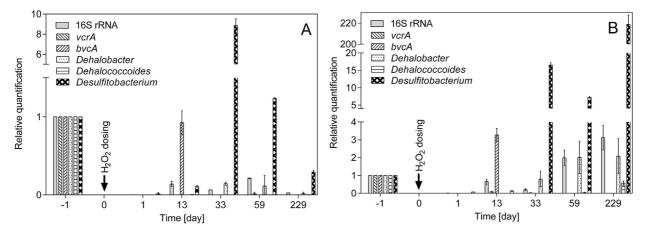
**Fig. 4.** Changes in the relative abundance of organohalide-respiring bacteria markers and 16S rRNA gene following application of hydrogen peroxide (500 L) in well RW5-12: A) depth 8 m, B) depth 13 m. Aside from the *Desulfitobacterium* (degrader of chloromethanes), no molecular genetic markers were identified one day after dosing. Note fragmentation of the y-axis.
