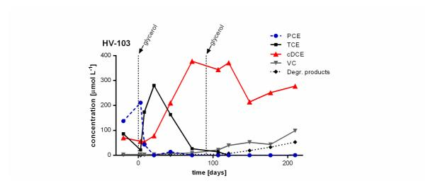
**Fig. 14.** Changes in the concentration of CEs and their final degradation products (the sum of ethene and ethane) following glycerol application in HV-103 well.
