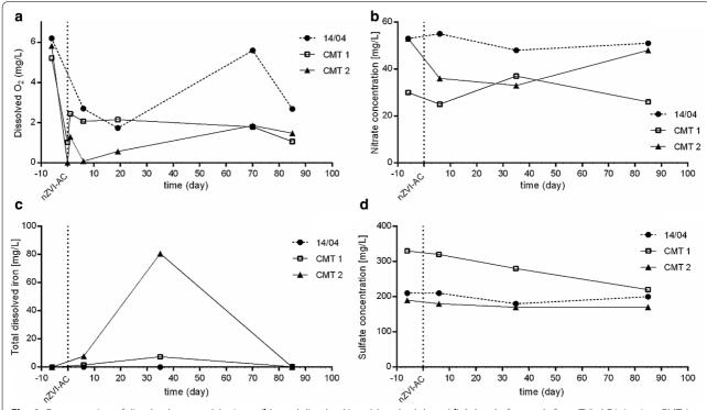
Fig. 4 Concentration of dissolved oxygen (a), nitrate (b), total dissolved iron (c) and sulphate (d) 6 days before and after nZVI–AC injection. CMT 1 and 2 = continuous multichannel wells, 14/04 = control monitoring well
