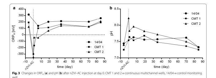
OH<sup>-</sup> [2]. The pH of both layers had dropped to the initial level of approximately 7.3 at the end of the study on day 85 (Fig. 3b). A similar pH trend to that in CMT 1 was also observed in groundwater from the upgradient well 14/04, indicating a temporal effect of nZVI–AC injection on groundwater in nearby upgradient areas (discussed further below).
