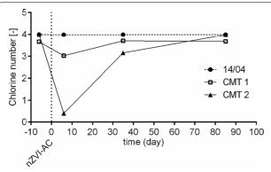
**Fig. 6** Changes in CI no. following nZVI–AC injection at day 0, calculated as the weighted average number of CI atoms per molecule of ethene
