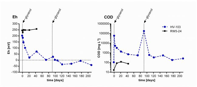
Fig. 1. Changes in Eh and COD in each well following glycerol injections. Note the logarithmic scale of the COD y axis.
