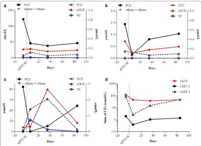
Fig. 5 Concentrations of CEs, ethene and ethane in groundwater from wells 14/04 (a), CMT 1 (b) and CMT 2 (c). Left axis represents PCE and the sum of ethene and ethane, while the right axis represents TCE, cDCE and VC. The sum of CE concentrations in a logarithmic scale (d)
