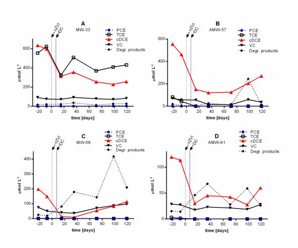
**Fig. 9.** Changes in the concentration of CEs and their final degradation products (the sum of methane, ethene, and ethane) following nZVI injection and direct current (DC) treatment. (A) reference well MW-33; (B) application well close to a cathode AMW-57; (C) monitoring well close to a cathode MW-58; (D) application well close to an anode AMW-61.
