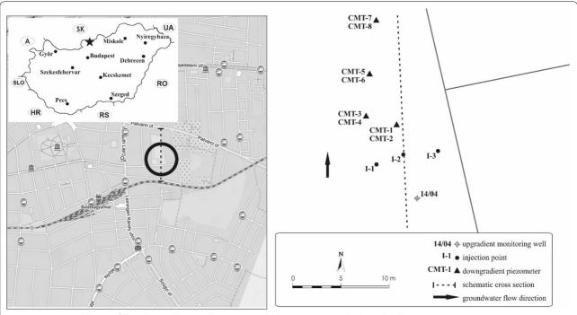
**Fig. 2** Location and layout of the pilot test area in Balassagyarmat. CMT = continuous multichannel wells, I = nZVI-AC injection points, 14/04 = control monitoring well. Schematic cross section shown in Fig. 1 is indicated by dashed line
