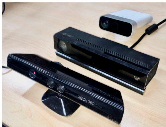
Obr. 3.3: Zľava doprava - Kinect v1, Kinect v2, Azure Kinect [17]
