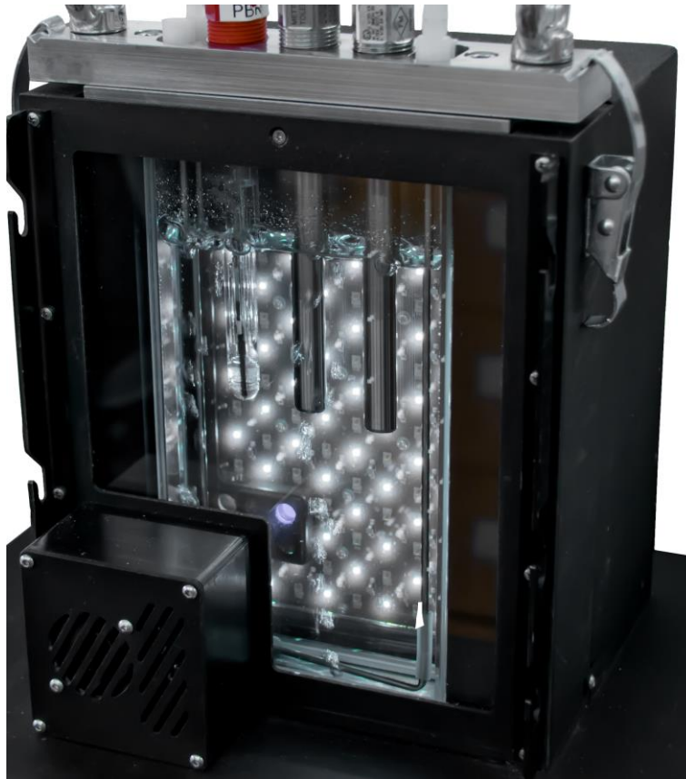
Figure 3.4 Cuvette illuminated from the back with a white LED array (PSI, 2021)
