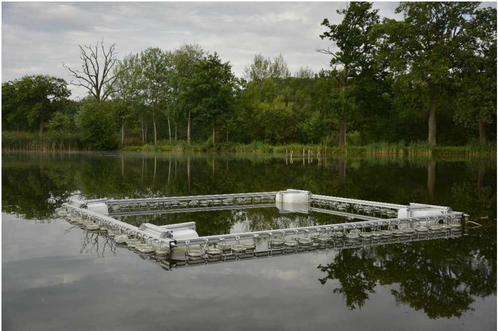
Figure 1: Field experiment construction and arrangement. The glass flasks were randomly hung up on floating aluminium square anchored to the bottom of the pond.
