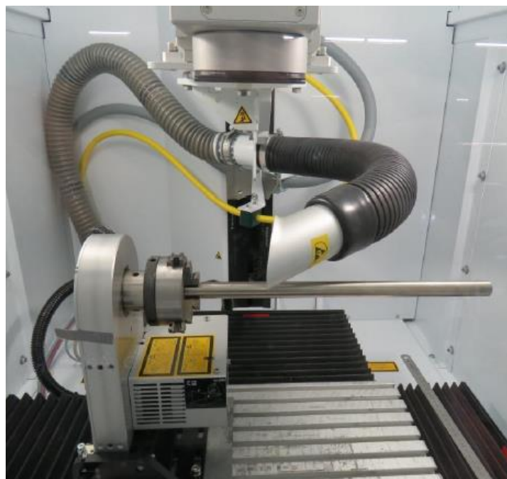
Obr. 5.14 TruMark Station 5000 s laserom TruMark 5050
