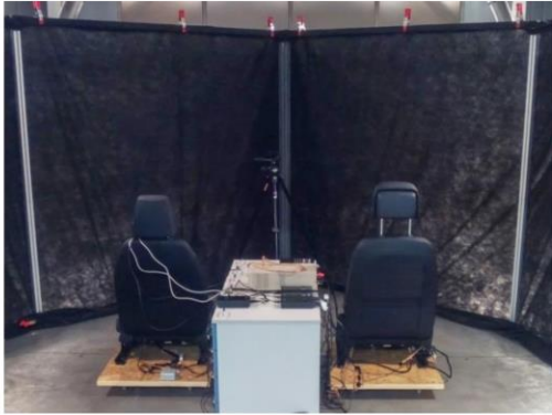
Figure 2 Experimental setup in the climatic chamber at BUT. Left – control/heated seat with textile upholstery. Right – ventilated seat with leather upholstery. Seats were placed in the geometrical centre of the chamber.
