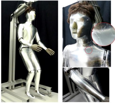
Fig. 1. Application of the low emissivity coating in detail.
