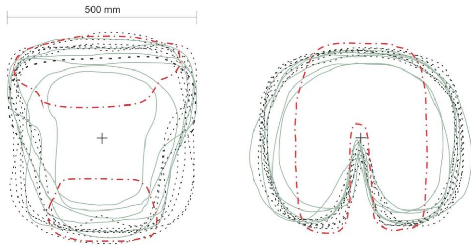
Fig 5. Centred shapes of the seat prints. Back prints (left) and buttocks prints (right). Dashed line indicates a subjects group with body weight of more than 80 kg, continuous line with less than 80kg, and red dotted line depicts the contact of the Western Newton type manikin.
