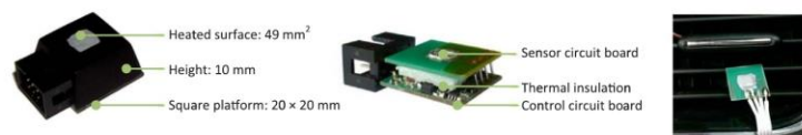
Fig. 3. Dimensions of the equivalent temperature sensor (left); insight into the sensor electronics (centre); application of the wired sensor into an HVAC vent (right).
