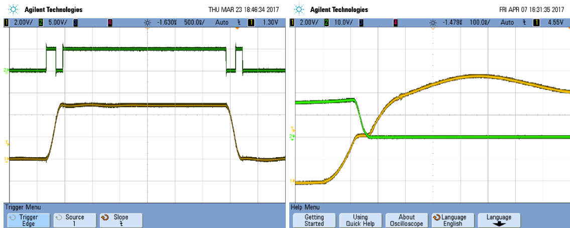
Fig. 95: Scope snapshot of recuperative gate driver during operation (left), Detuning effect of Miller capacitance (right)
