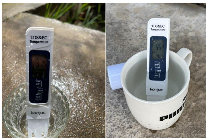
Figure 8 Measurement of pH, TDS, electrical conductivity EC, and temperature in the field
