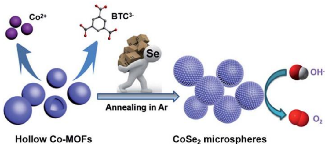
Figure 22. Schematic illustration of the synthetic strategy of the CoSe 2 Microspheres. Taken from Ref. 89 and modified.
