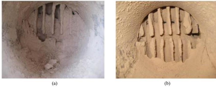
Figure 2: Actual pattern of ash deposition on H-type finned tube heat exchanger at different gas velocities after 18 hours at flue gas velocities (a) 4.5 m·s-1; (b) 6.25 m·s-1, for gas with high ash content. [2, p. 4683]
