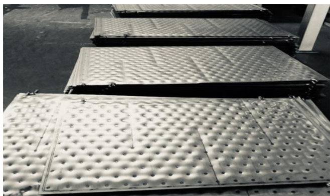
Figure 6: Flue Gas Heat Exchanger Welded Pillows [4]
