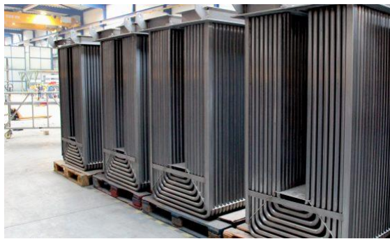
Figure 3: Flue gas heat exchanger [3]
