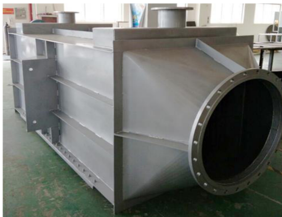
Figure 5: Flue Gas Heat Exchanger [4]
