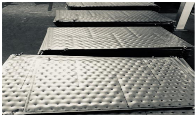
Figure 6: Flue Gas Heat Exchanger Welded Pillows [4]
