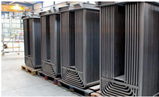
Figure 3: Flue gas heat exchanger [3]
