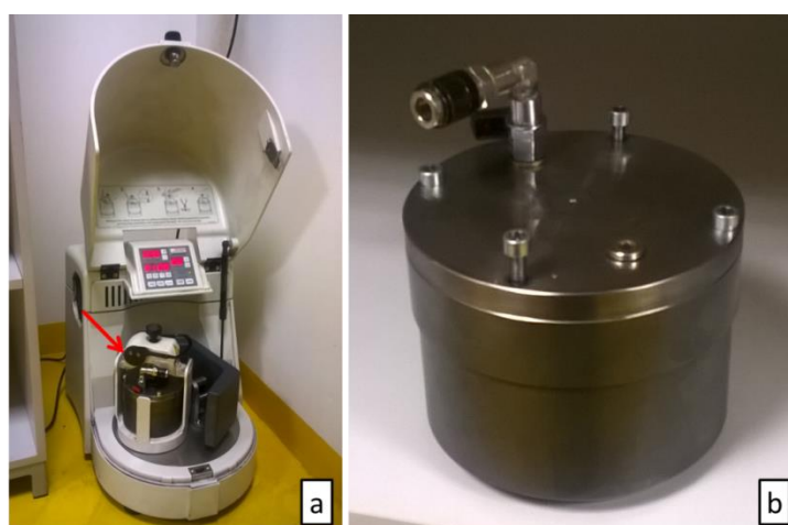
Fig. 41 - Ball milling equipment a) planetary ball mill Fritsch Pulverisette 6 (milling bowl denoted by red arrow) b) detail of milling bowl.
