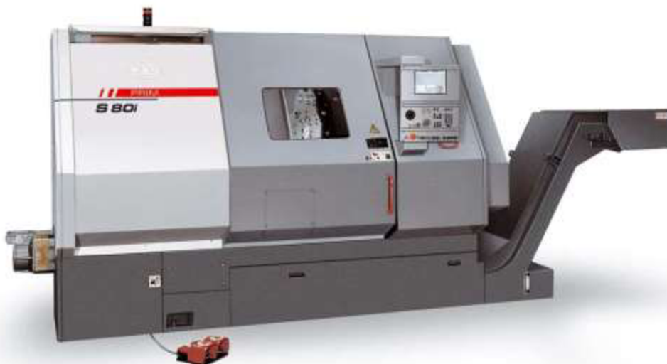
Obr. 3.2 – Soustruh MAS S80i [19].
