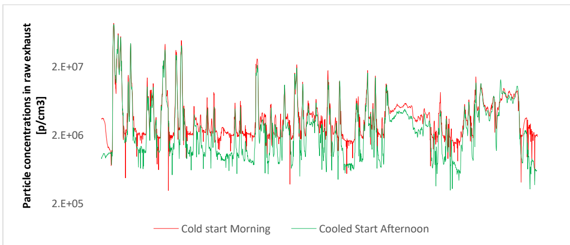
Figure 5. 19 Particle concentration comparison in engine exhaust between morning cold start and afternoon cooled start
