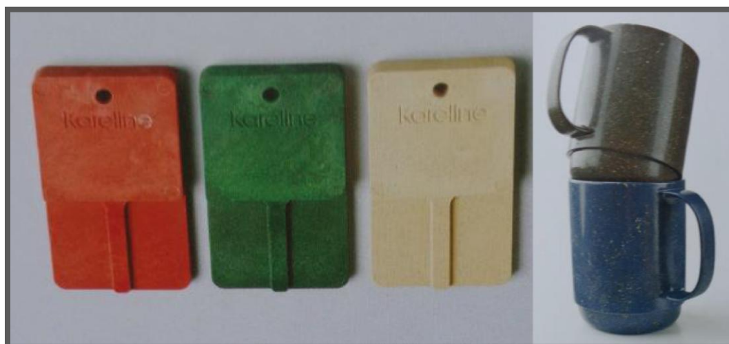
Obr. 5-18 Termoplast PLMS 6040 a AgriResin [74]
