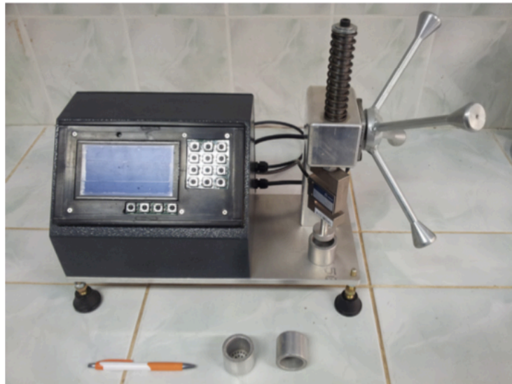
Figure 9: Mud press machine used by Kayabali et al., (2016).
