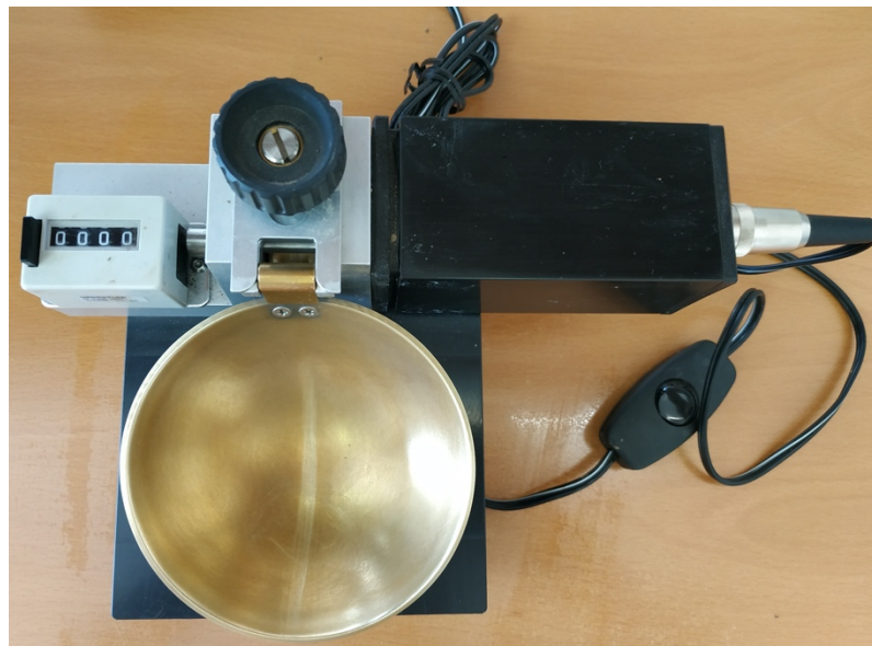
Figure 17: Casagrande apparatus after setting up and calibration, ready for experiment.
