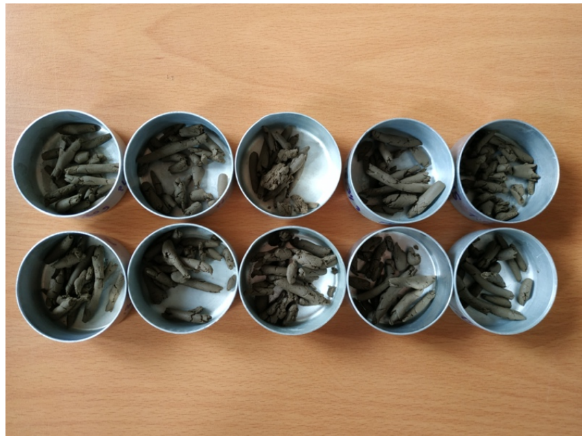
Figure 16: Plastic limit determination by rolling thread method (top) and soil samples after reaching their plastic limit, resulting in their disintegration into smaller pieces (bottom).
