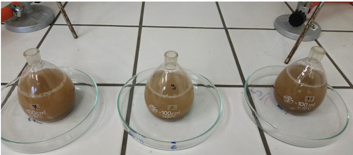
Figure 12: Pycnometers with boiled soil sample and water – water pycnometer method.
