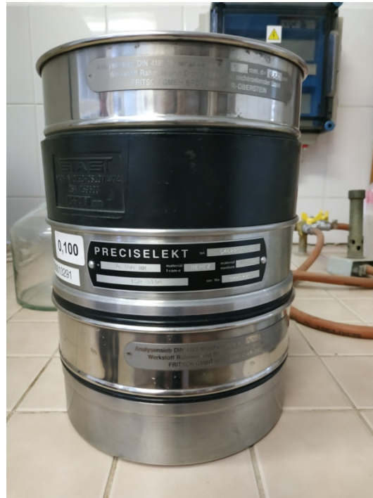
Figure 14: Four sieves with different diameters (1, 0.5, 0.1 and 0.063 mm) placed on top of each other, so that soil can be passed through them.
