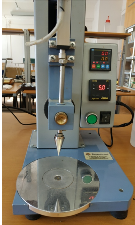
Figure 19: Cone penetrometer after setting up and calibration, ready for experiment.
