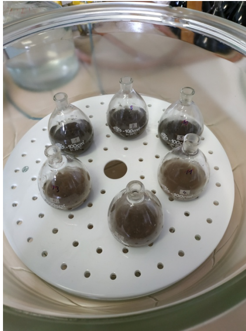
Figure 11: Pycnometers with soil samples and distilled water ready for vacuuming.
