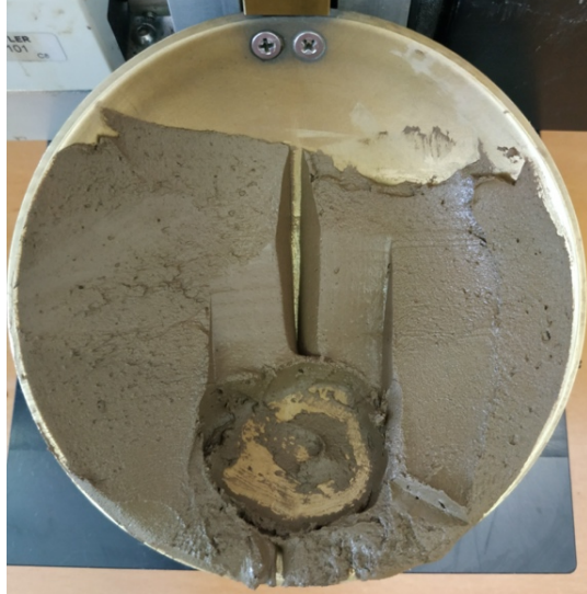
Figure 18: Experiment with Casagrande apparatus: smoothed soil on Casagrande cup (top left), cut-out groove (top right), taken-out soil around the closed groove (bottom).
