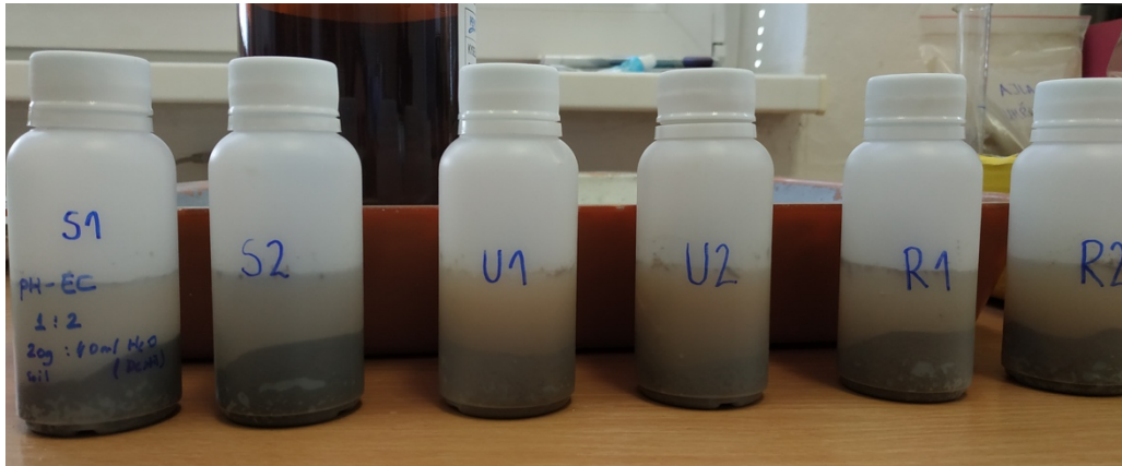
Figure 15: Soil samples inside plastic bottles ready for pH and EC analysis.
