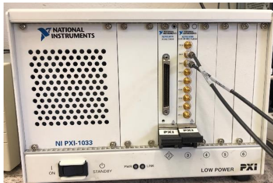
Figure 3-3. NI PXI chassis with oscilloscope.
