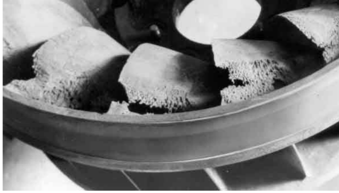
Figure 1-5. Cavitation damage on the blades of a Francis turbine [13].
