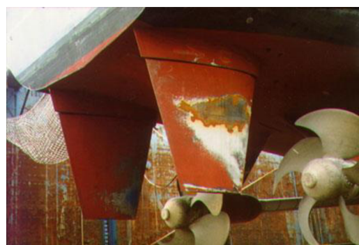
Figure 1-4. Cavitation effects on the rudder of a ship.
