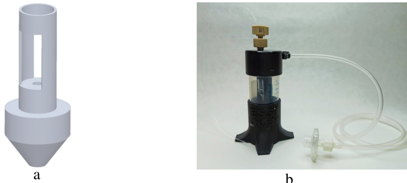
Fig. 4.5: In-house made reservoir for droplet reinjection; a - PC model of vial holder; b - Reservoir assembly used in the lab.
