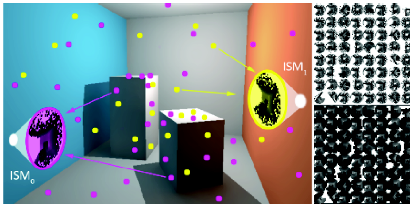
Figure 3.22: Illustration of ISMs concept. Simplified shadow maps (right,top) and interpolated after pull-push(right,bottom) [33]
