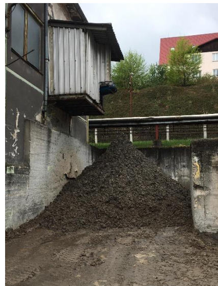
Figure 10: Dewatered pile of residues after water treatment in JIP Větrní (Author 2020).
